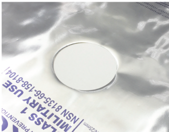
Step 1: Cut hole in packaging material.
