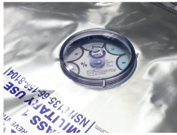
Step 2: Position Window housing in cut out
